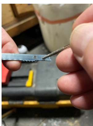
Left: Blade blank with teeth filed down and rivet holes drilled. Center: filing the rivet holes for test fitting. Right: Test fitting the rivets.
