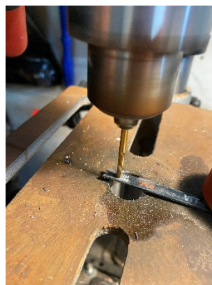
Left: Whittling blade stock, also known as Jigsaw blades. Center: Filing down the teeth. Right: Drilling the rivet holes.
