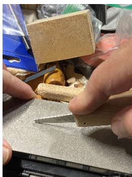
Left: Shaping the back side of a blade on a Sharpal 325 grit diamond stone. Center: A flat metal file can also be used. Right: rough shaping the bevel with flat file.
