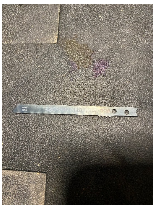
Left: Blade blank with teeth filed down and rivet holes drilled. Center: filing the rivet holes for test fitting. Right: Test fitting the rivets.
