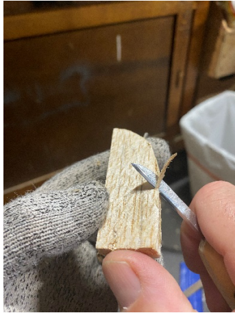
Left: Rounding the scabbard. Center: Scabbard rough carved and ready for sanding. Right: After sanding, burning in flat diamond gripping surface to match knife handle.
