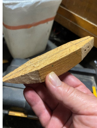
Left: Centerline and taper lines drawn on belly of handle. Center: Center line and taper lines drawn on back of handle. Right: Tapers boasted in.
