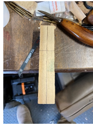
Left: Drilling the rivet holes in the handle blank. Center: Rivet holes drilled and back of tang marked. Right: Centerline and tang mark drawn.
