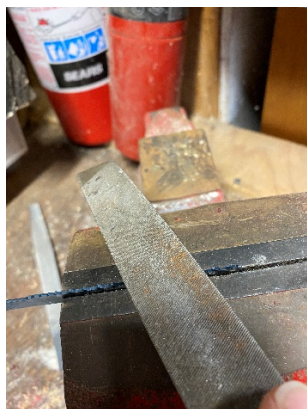
Left: Whittling blade stock, also known as Jigsaw blades. Center: Filing down the teeth. Right: Drilling the rivet holes.
