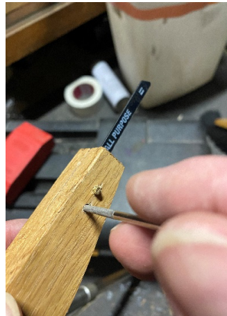
Left: Blade fitted into handle and first rivet test fitted. Center: Cleaning rivet hole before test fitting. Right: Rivets and blade blank successfully fitted to handle
