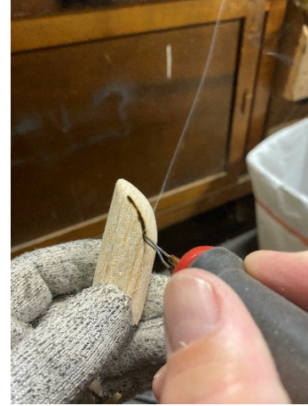
Left: Rounding the scabbard. Center: Scabbard rough carved and ready for sanding. Right: After sanding, burning in flat diamond gripping surface to match knife handle.
