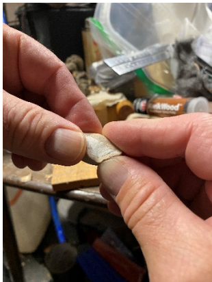
Left: Cutting the Kwikwood. Center: Kneading the putty. Right: pushing the putty into the kerf with the knife blank.
