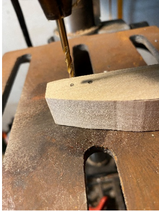
Left: Drilling the rivet holes in the handle blank. Center: Rivet holes drilled and back of tang marked. Right: Centerline and tang mark drawn.
