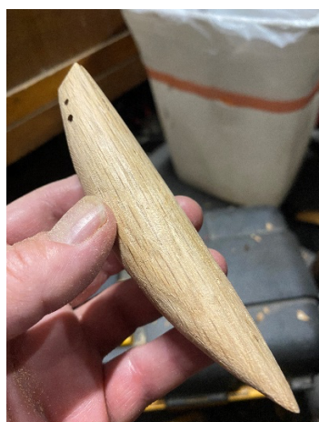
Left: Smoothing out tool marks with flat wood file. Center: Handle with tool marks removed. Right: Sanding out the file marks.
