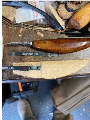
Left: Drilling the rivet holes in the handle blank. Center: Rivet holes drilled and back of tang marked. Right: Centerline and tang mark drawn.
