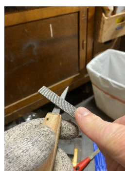
Left: Shaping the back side of a blade on a Sharpal 325 grit diamond stone. Center: A flat metal file can also be used. Right: rough shaping the bevel with flat file.
