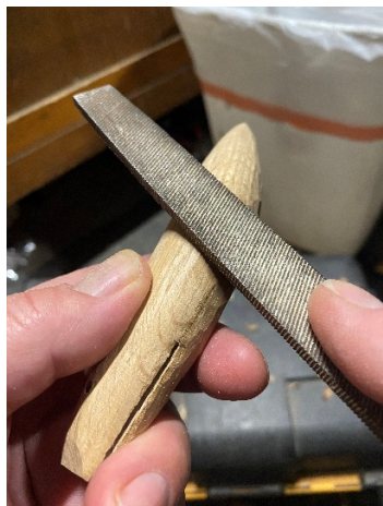
Left: Smoothing out tool marks with flat wood file. Center: Handle with tool marks removed. Right: Sanding out the file marks.
