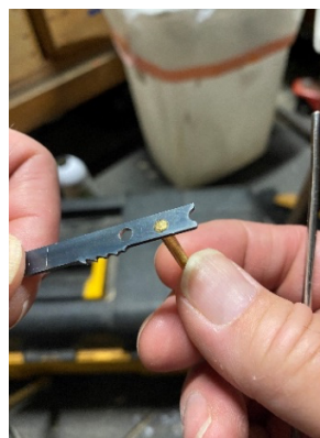
Left: Blade blank with teeth filed down and rivet holes drilled. Center: filing the rivet holes for test fitting. Right: Test fitting the rivets.
