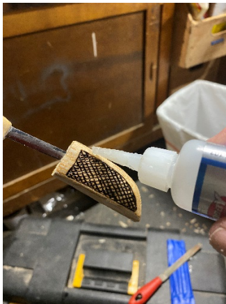
Applying cyano-acrylate glue to seal and finish the scabbard.
