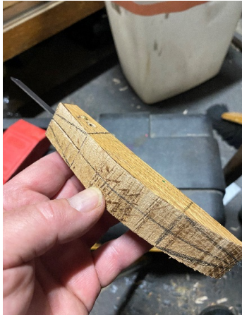
Left: Centerline and taper lines drawn on belly of handle. Center: Center line and taper lines drawn on back of handle. Right: Tapers boasted in.
