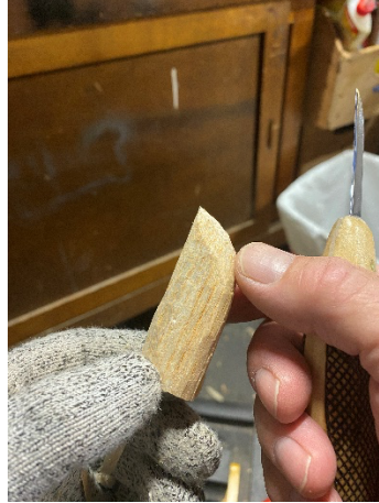
Left: Rounding the scabbard. Center: Scabbard rough carved and ready for sanding. Right: After sanding, burning in flat diamond gripping surface to match knife handle.
