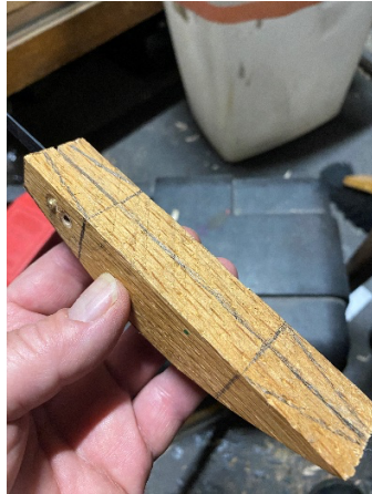
Left: Centerline and taper lines drawn on belly of handle. Center: Center line and taper lines drawn on back of handle. Right: Tapers boasted in.
