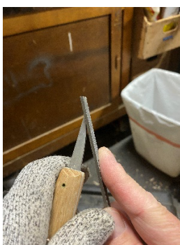
Left: Shaping the back side of a blade on a Sharpal 325 grit diamond stone. Center: A flat metal file can also be used. Right: rough shaping the bevel with flat file.
