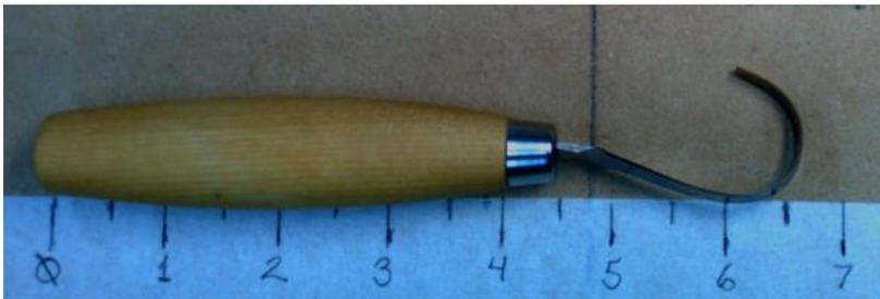
**Sloyd knife** - Used in flat plane carving, a single knife to carve many things, fancy whittling. Sloyd is not a person or place name. It is derived from a Swedish word meaning handiwork or crafts. The manufacturer is Morakniv, and the price is \$30.
