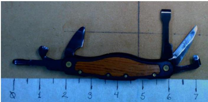
**Whittlers pocket knife** - A folding knife with two or more blades, commonly used for whittling. I use two, a three bladed folding knife and a two bladed one. Very good for casual carving. –
