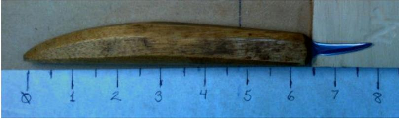
**Cottonwood bark knife** – This knife is designed to carve cottonwood bark. For this purpose, it has a rounded end with no point to prevent rip-outs. The edge follows most of that rounded end. The manufacturer is Gil Drake, and the price is \$45-\$50.
