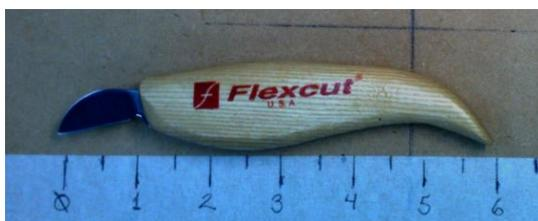
**Detail knife** – This knife has a thin curved blade, and is used for detail finishing work. Manufacturer is Tom Wolfe, collectors item, hard to price
